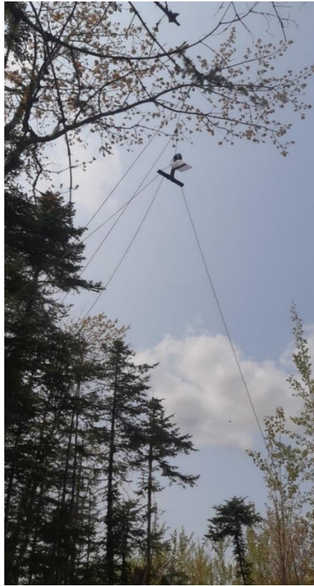
FIGURE 2. PHOTOS OF THE TWO ACOUSTIC MONITORING STATIONS SHOWING ELEVATED MICROPHONE POSITIONS WITH WEATHERPROOF SOUND DEFLECTING APPARATUS.
