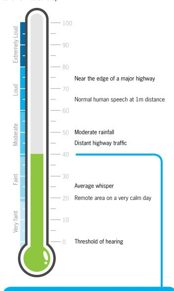
At a distance of 550 metres, typically the sound from a wind turbine will have a sound pressure level of approximately 40 decibels at the outside of a residence.
