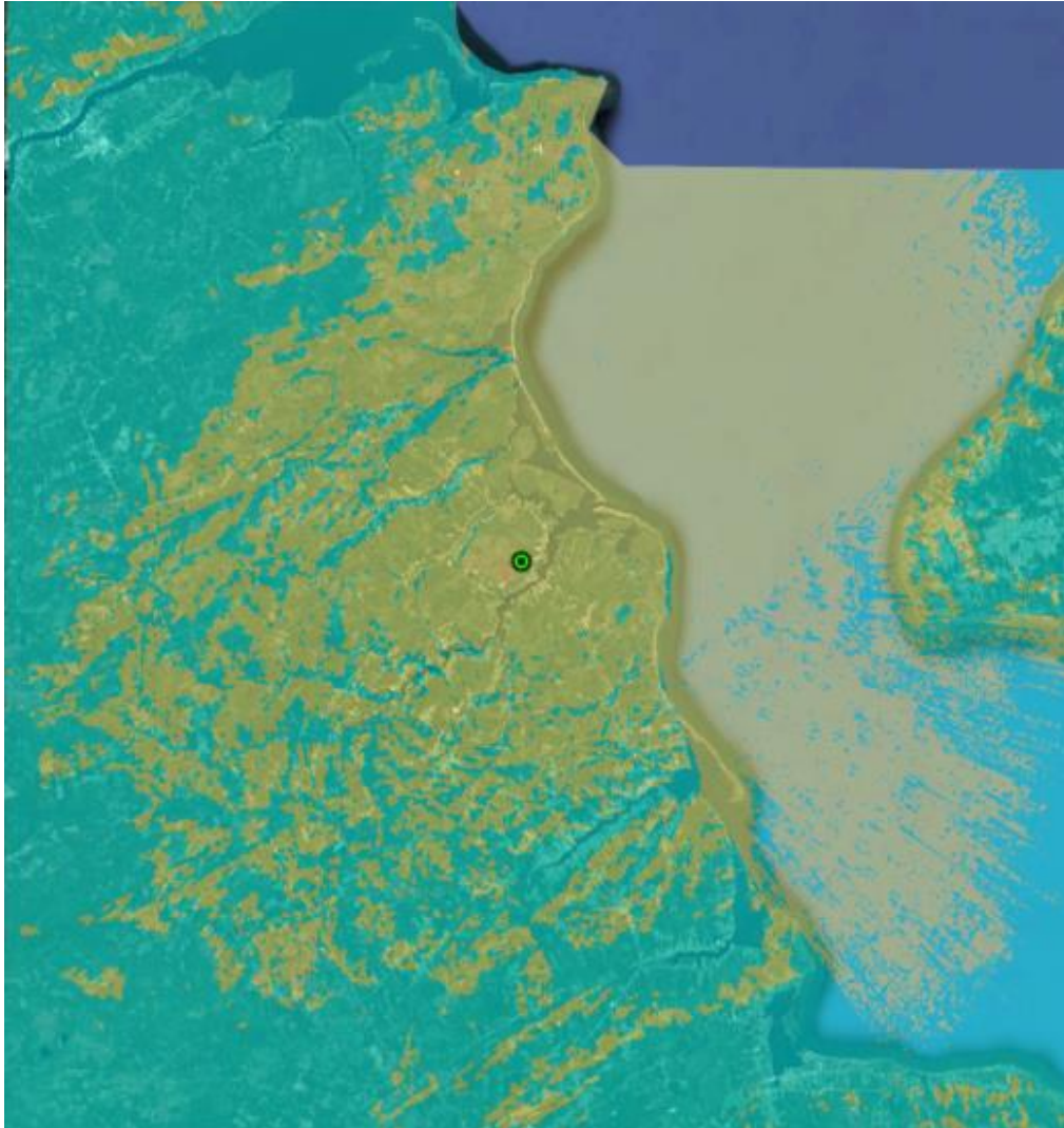
Figure 5-5: Zone of Visual Influence over a 48km visual analysis radius. Yellow color demonstrates some portion of the turbine may be visible.
