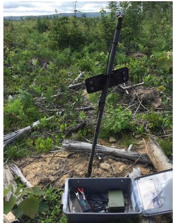
Photo 2: Wildlife Acoustics SM4BAT ultrasonic bat detector and condenser microphone used at station 1.
