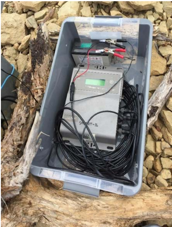
Photo 1: Wildlife Acoustics SM3BAT detector used at Station 3.
