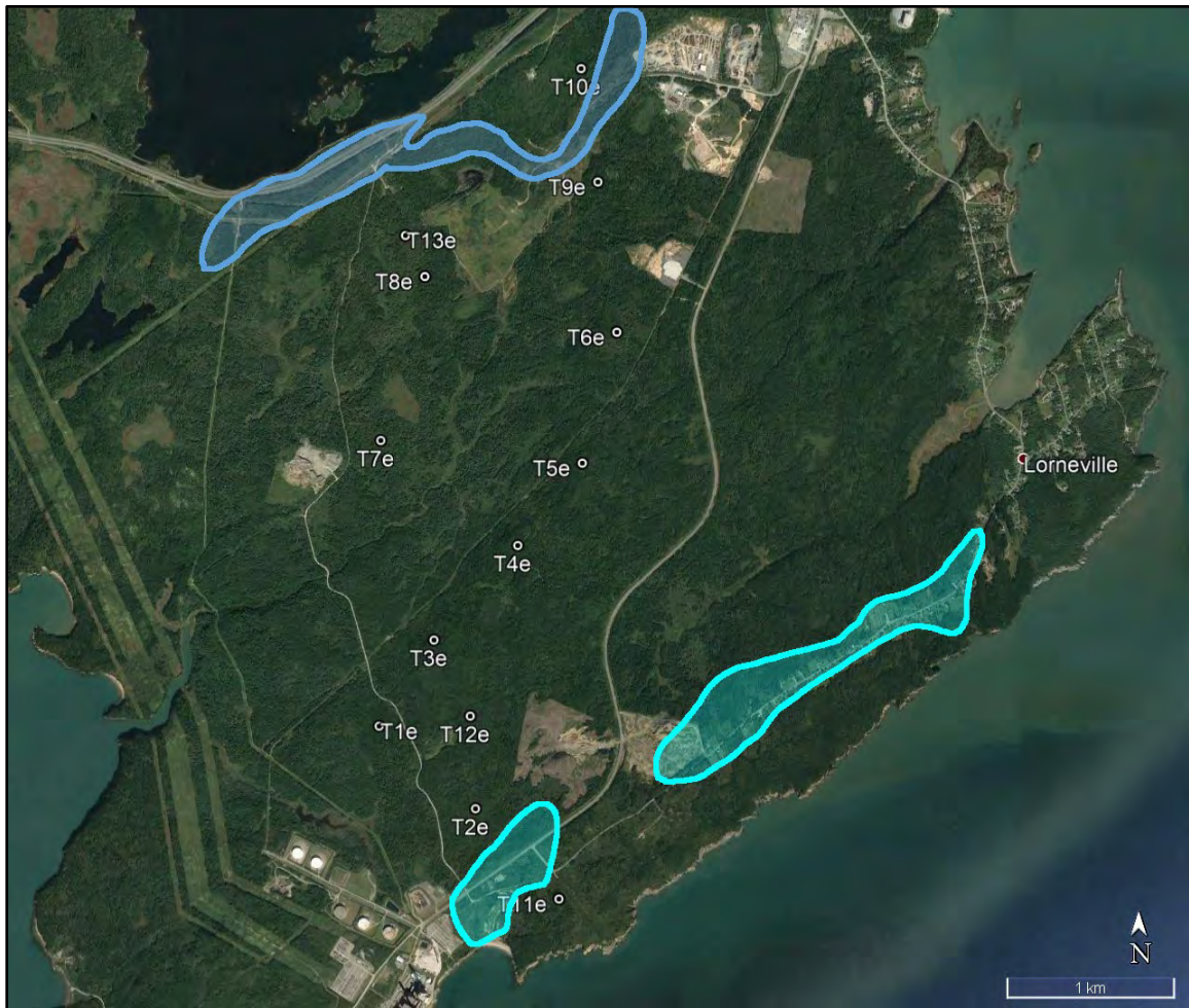
Figure 4: Project area on a satellite image with turbine locations & geology. The southern deposits are 'marine shallow water deposits', and the northern deposit is a 'ice contact stratified drift'.
