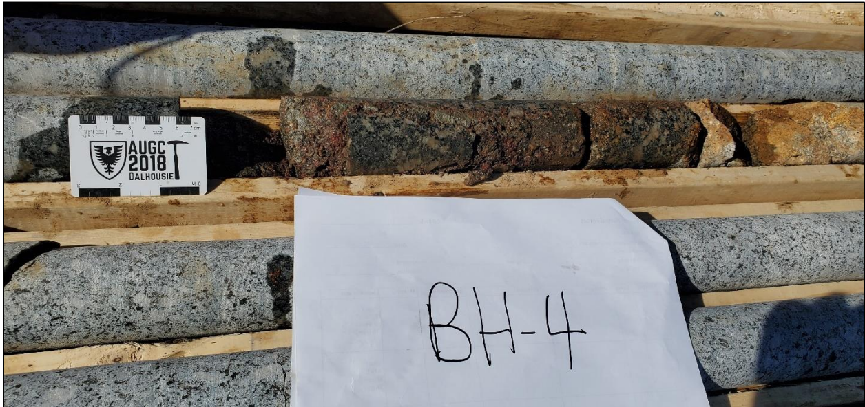
Figure 20: Weathering and alteration along a fracture zone in borehole BH4 at proposed turbine site T15 - ~ 6.7 m (22 ft) depth.
