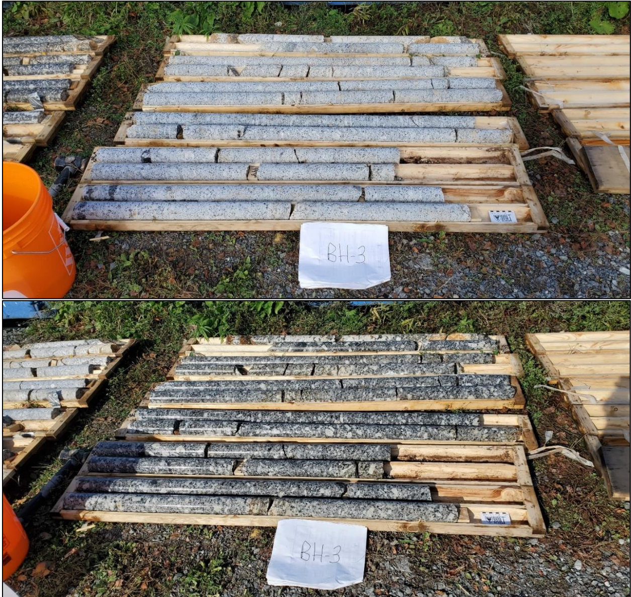
Figure 17: (Top) Photograph of dry borehole BH3 core from proposed turbine location T14, with core boxes organized by depth – top in upper left. (Bottom) Duplicate photograph of BH3 core, wet. Light grey, coarse-grained biotite monzogranite with large plagioclase megacrysts predominates.
