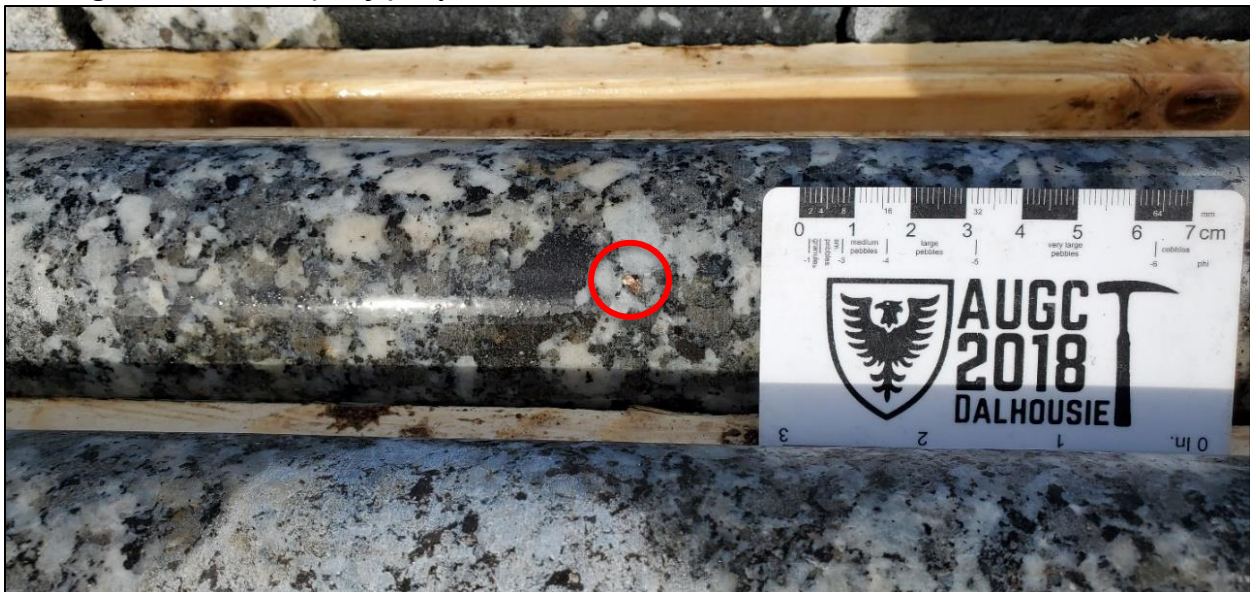
Figure 22: Example of a 3-5mm weakly magnetic pyrrhotite grain in Salmontail Lake Monzogranite - ~ 2.5m (8.2 ft) depth.
