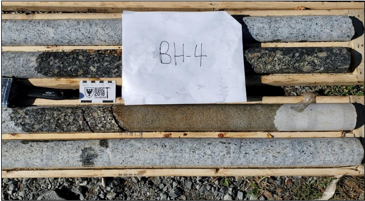
Figure 21: Sharp contact between Salmontail Lake Monzogranite and the greyish-pink Gold River Leucomonzogranite in borehole BH4 at proposed turbine site T15 - ~14.5m(47.5 ft) depth
