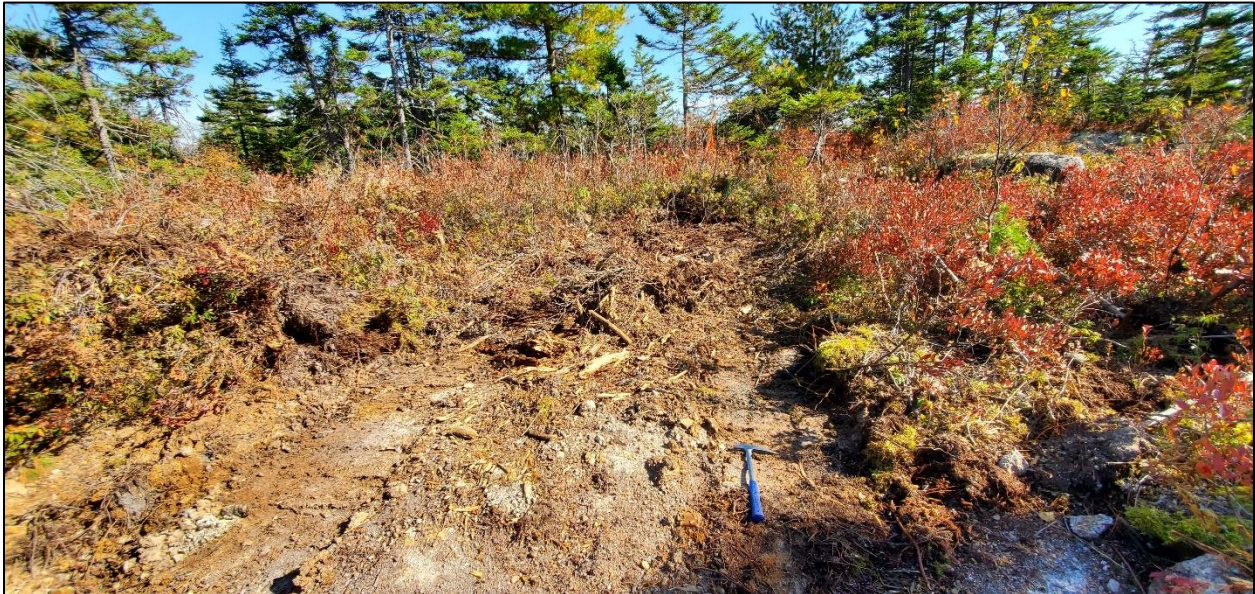
Figure 12: Photograph of a backfilled-excavated test pit filled with brown soil and large granite cobbles. Adjacent boulders can be seen and are comprised of coarse-grained biotite granite. This site had a background gamma radiation level of 234 cps.
