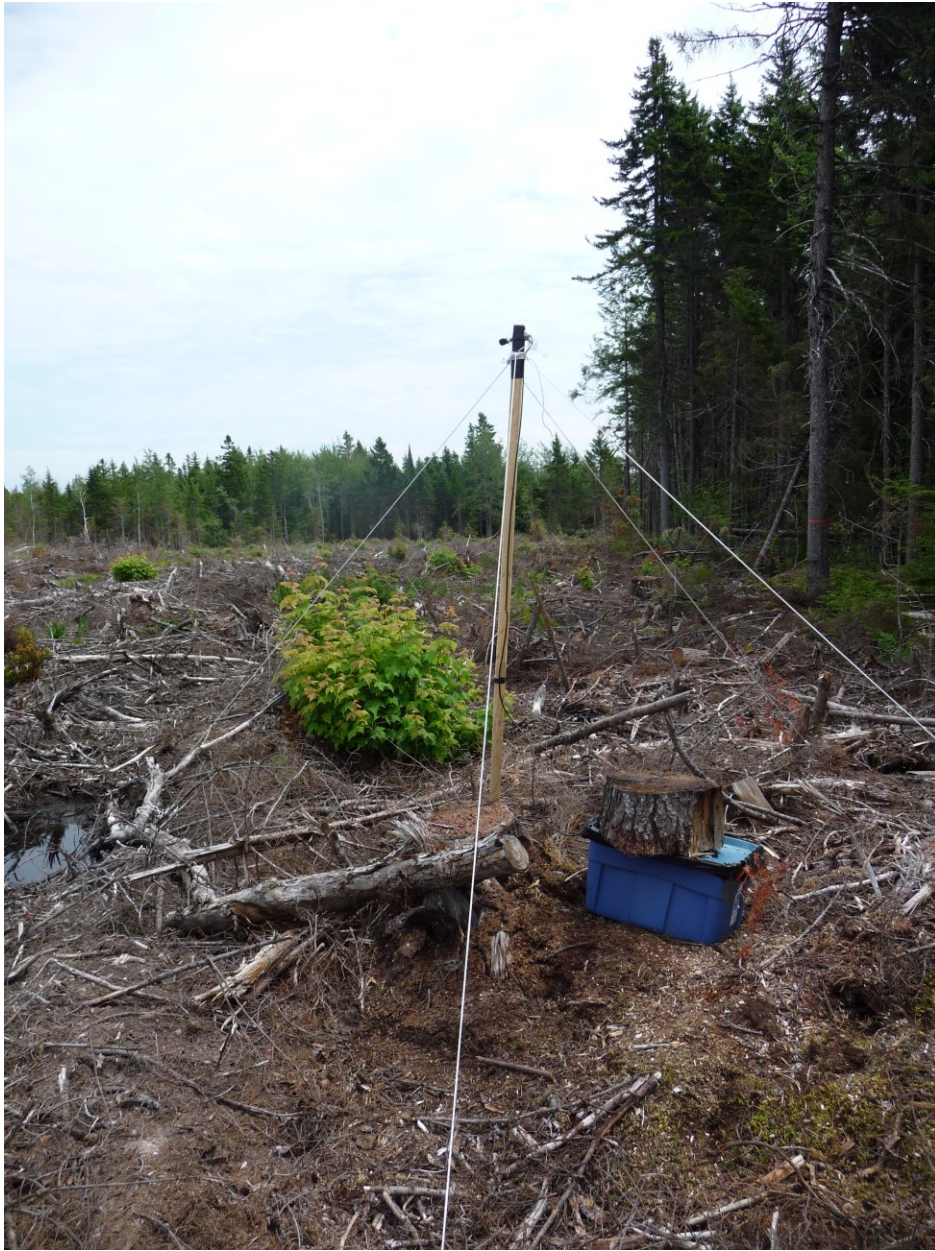
Figure A4. Bat detector (SM2Bat+) placement at site 4 along a forest edge.
