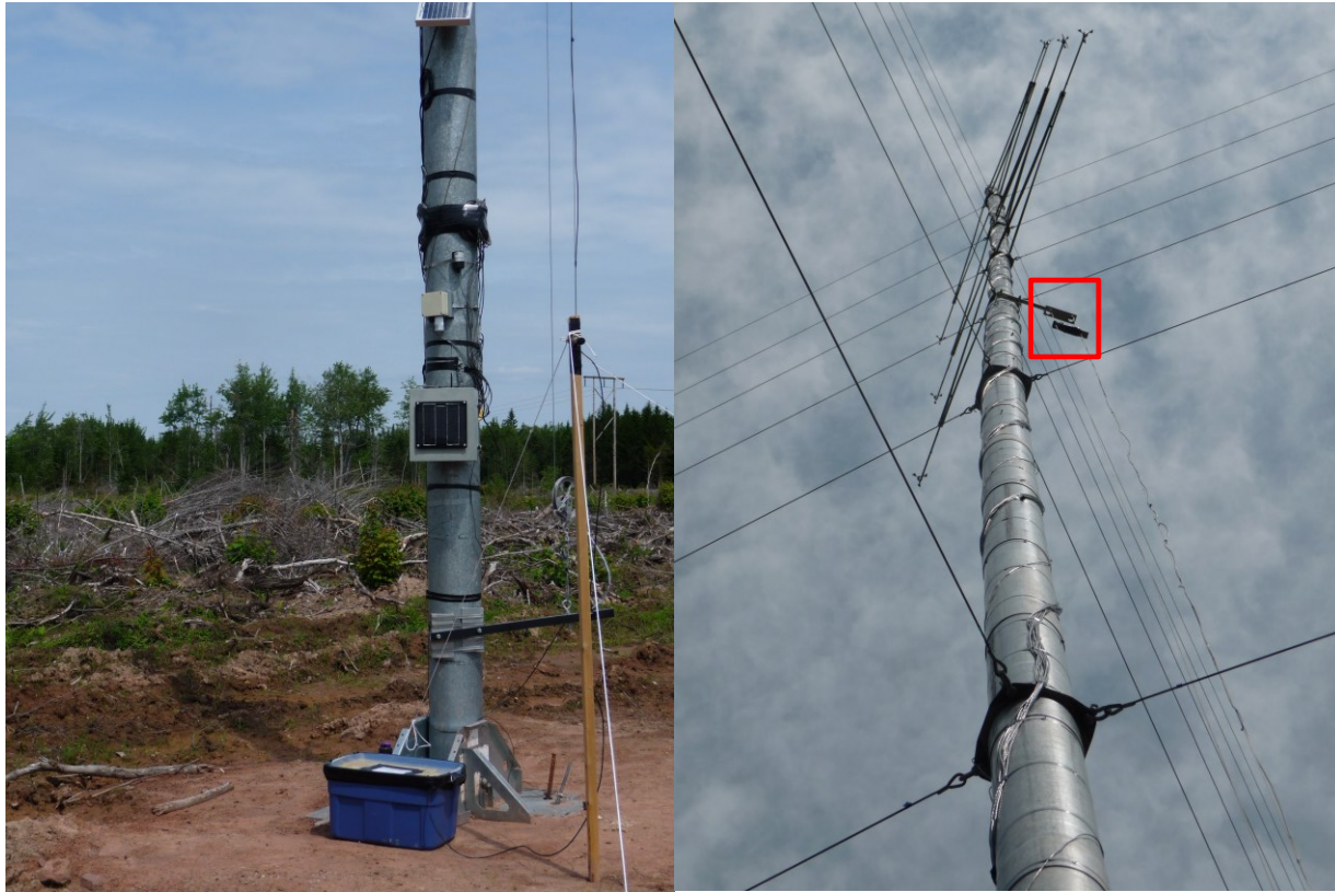
Figure A2. Bat detector (SM2Bat+) placement at site 2 showing the low microphone on the 2x2 (2 m AGL). Red rectangle shows the high microphone position on the MET tower ( \approx 33 m AGL).
