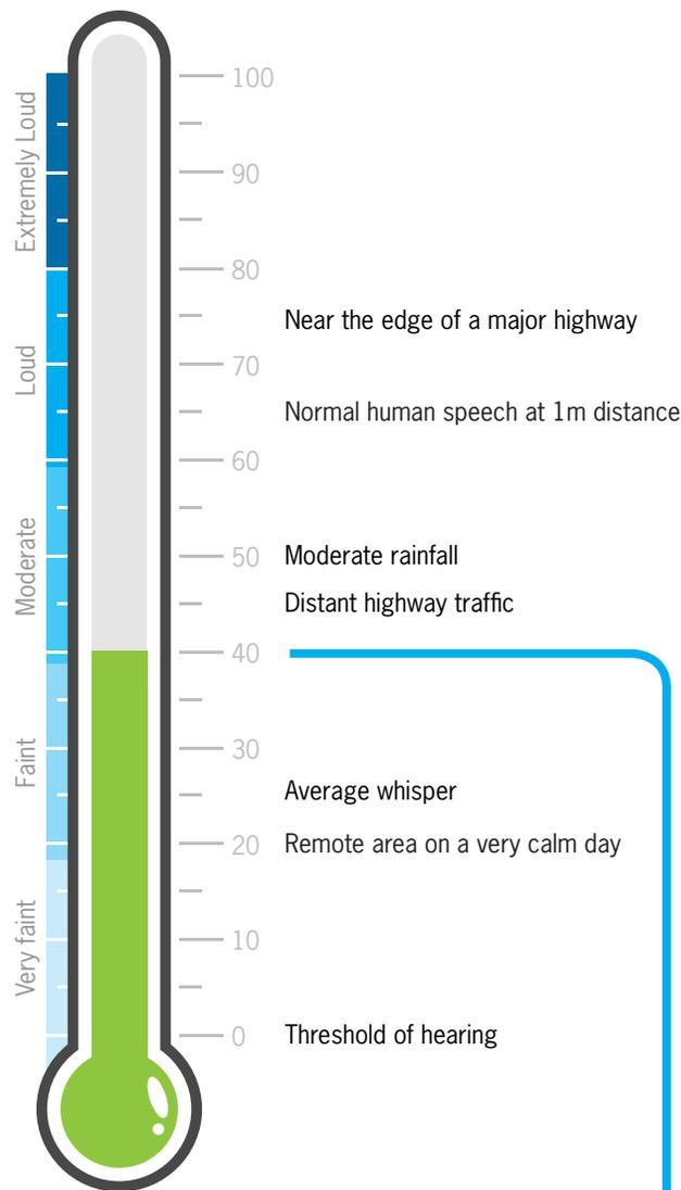
At a distance of 550 metres, typically the sound from a wind turbine will have a sound pressure level of approximately 40 decibels at the outside of a residence.
